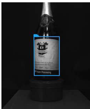
Results of applying RemapImage with a spatial map created with the CreateCylinderMap filter.
