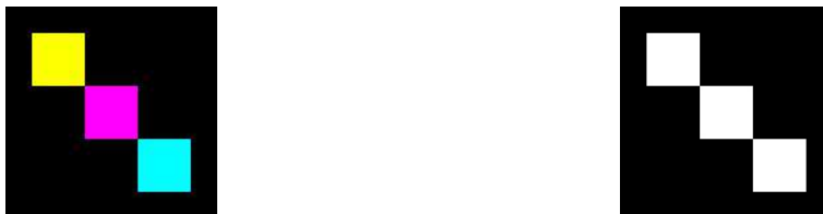
Input RGB image (on the left) converted to single-channel image (on the right) with pixel values obtained from summing with saturation values of input image channels. In the picture on the left-hand side, pixel values in the colorful squares are {255, 255, 0}, {255, 0, 255} and {0, 255, 255}, and their type is UInt8. After addition with saturation, values of corresponding pixels in the output image will be {255} - because maximal value for UInt8 pixels is 255 and \min(255 + 0 + 255, 255) is 255.
