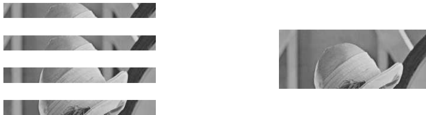
JoinImages used to join multiple image stripes into a single image.
