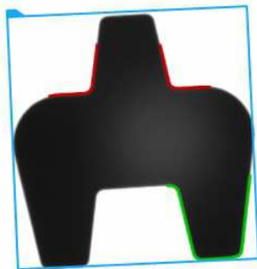
Object location found based on two matching objects (red and green).
