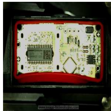
The SubtractFromImage performed on the sample image with inValue = 50.0.
