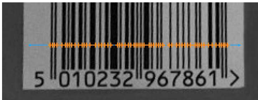
ScanExactlyNEdges locates the edges using a scan map representing the scan path above ( inEdgeCount = 61).
