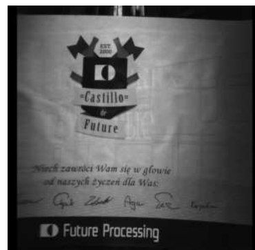
Results of applying RemapImage with a spatial map created with the CreateCylinderMap filter.
