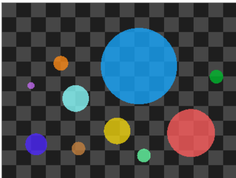
GetMinimumRegion performed with Area as the selected region feature.
