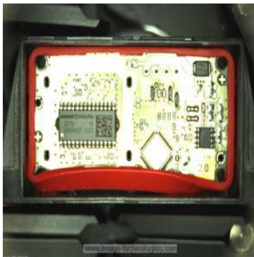
AverageChannels_Weighted run on example image with inWeight1 = 1, inWeight2 = 0, inWeight3 = 0, inWeight4 = 0, which for a RGB image is equivalent to the extraction of the Red channel.
