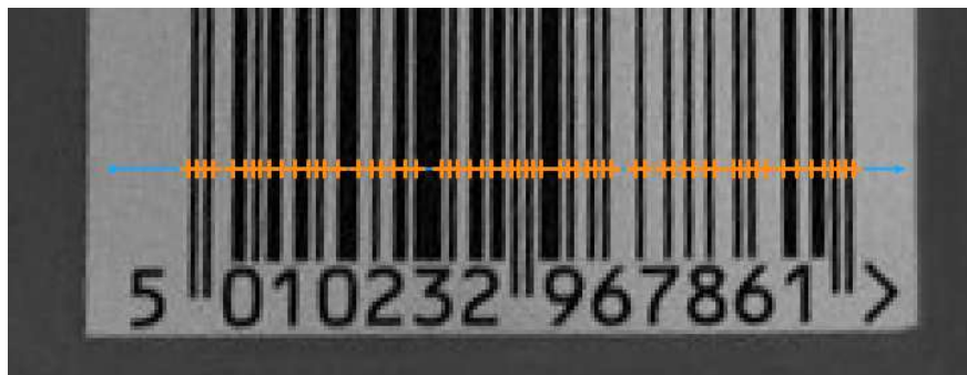
ScanExactlyNEdges_Direct locates the edges across inScanPath ( inEdgeCount = 61).
