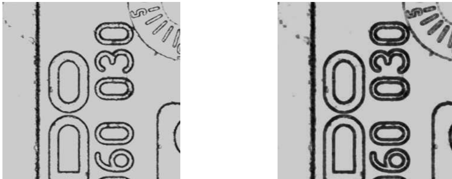
ErodeImage performed on the sample image with inKernel = Box, inRadiusX = 1, inRadiusY = 1.
