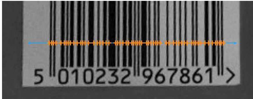
ScanExactlyNEdges_Direct locates the edges across inScanPath .
