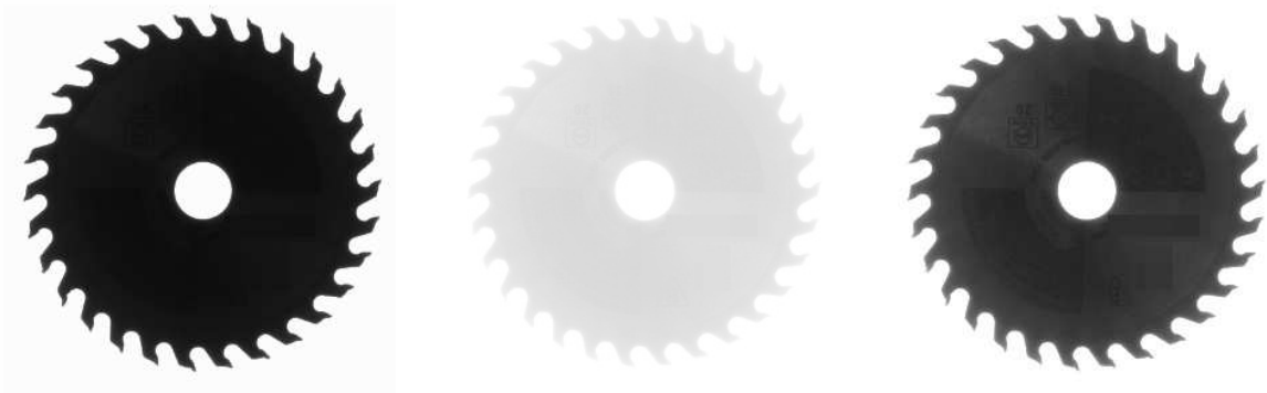
The LogarithmImage performed on the sample image with parameters inScale = 250, inOffset = 50. The middle image inNormalizeZero = False and the left image has inNormalizeZero = True .
