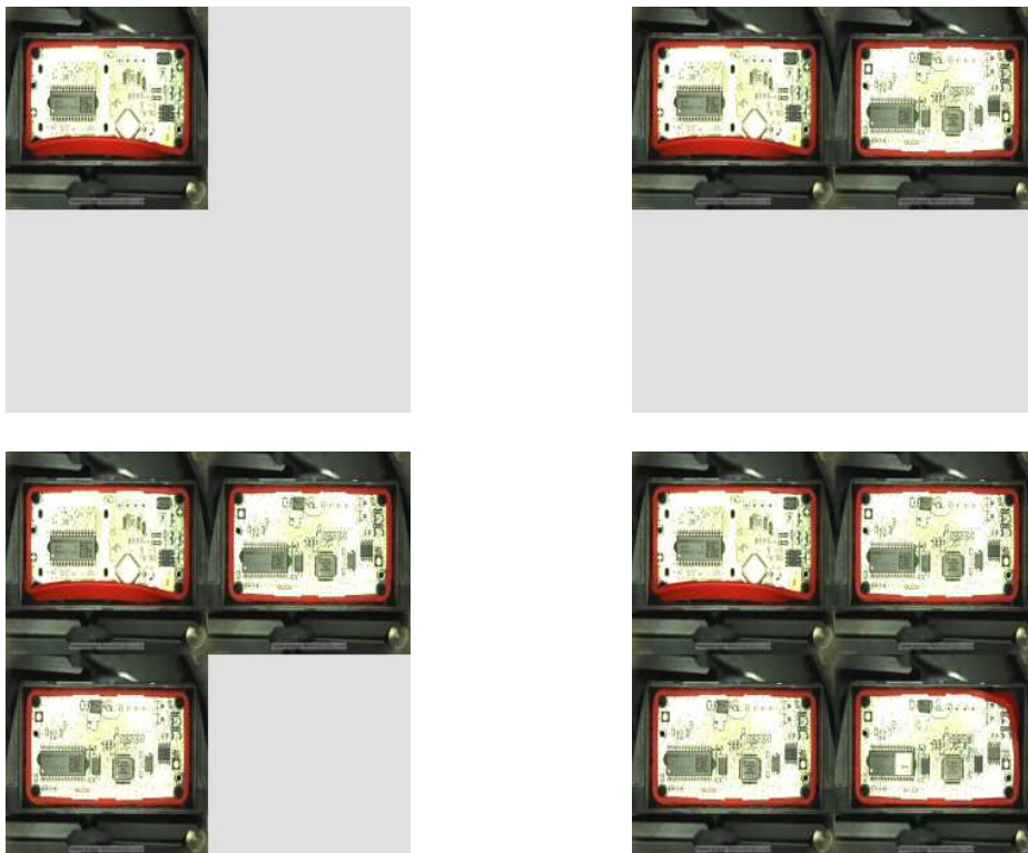
Four consecutive instances of the DrawGridImage used to plot an image grid. Each of the filters receives different inImage and different pair of the inColumnIndex , inRowIndex parameters - accordingly: (0,0) (0,1) (1,0) (1,1).
