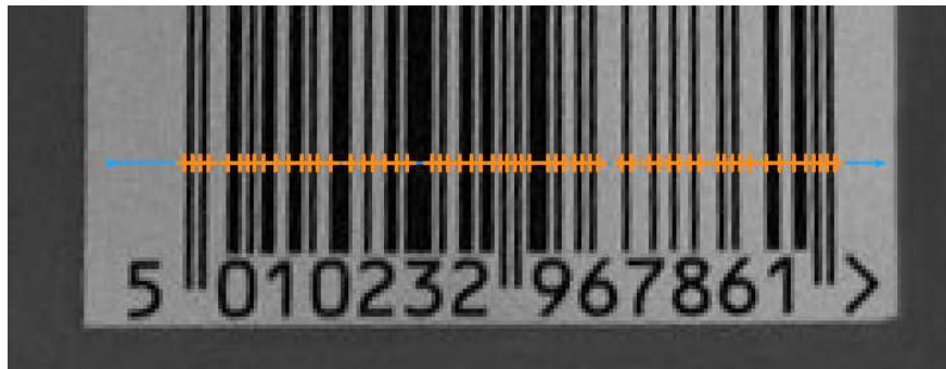
ScanExactlyNEdges locates the edges using a scan map representing the scan path above.
