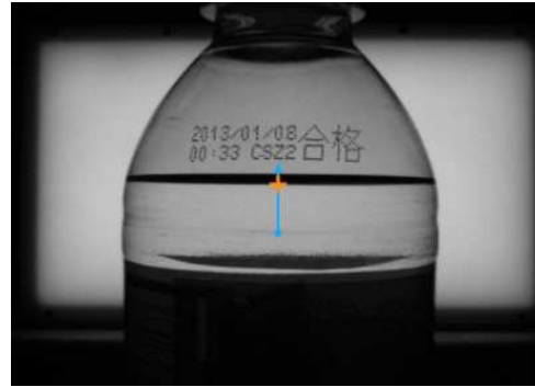
ScanSingleEdge_Direct locates the strongest edge across inScanPath.
