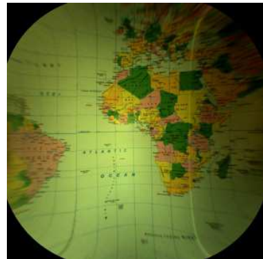
Results of applying RemapImage with a spatial map created with the CreateSphereMap filter.
