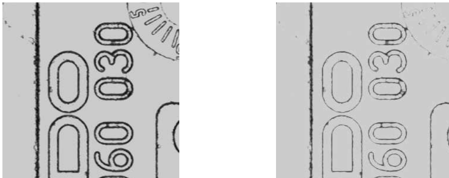
DilateImage performed on the sample image with inKernel = Box, inRadiusX = 1, inRadiusY = 1.
