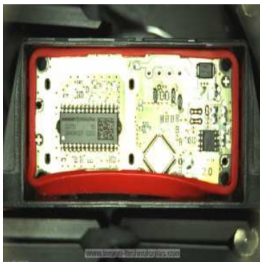
The SubtractFromImage performed on the sample image with inValue = 50.0.
